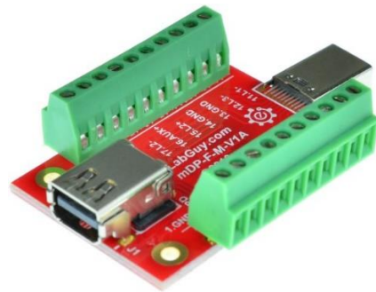
Figure 4: mDP-F-M-V1A with terminal blocks
